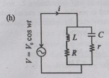
Find the resonance frequency of the circuit.
