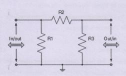
ii) Draw equivalent T-network of the above  $\pi$  network where  $R_1$ =5 ohm,  $R_2$ =3 ohm and  $R_3$ =4 ohm (Marks: 4)
